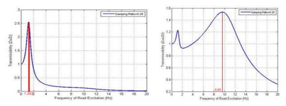
Figure 3: QFRCo Sprung Mass Transmissibility Figure 4: QFRCo Unsprung Mass Transmissibility
