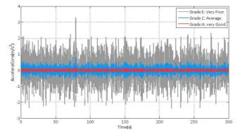
Figure 11: QFRCo Sprung Mass Accelerations: Random: Effect of Road Grades
