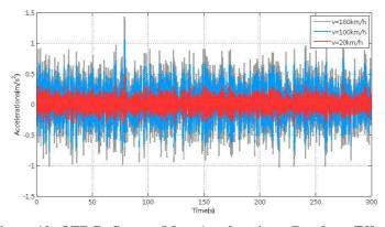
Figure 12: QFRCo Sprung Mass Accelerations: Random: Effect of Speed
