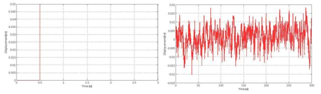
Figure 2: Input Road Disturbances Modeled as Discrete and Random Events
